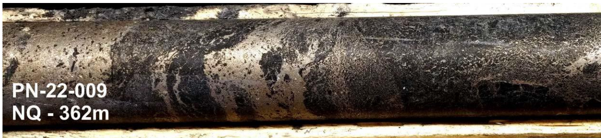
Figure 7.7 - Semi-massive pyrrhotite beds
