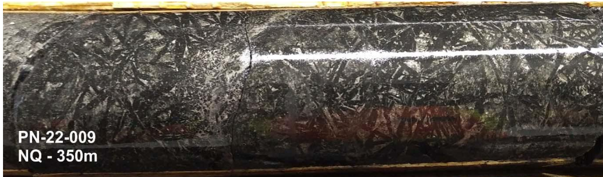
Figure 7.8 - Matrix sulphides with olivine needles
